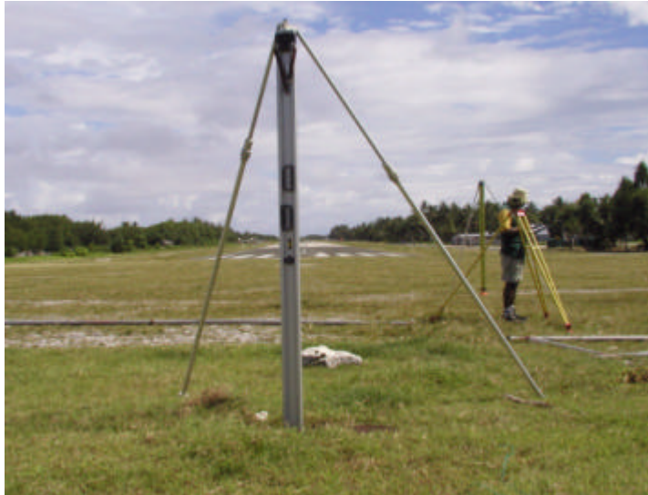
Levelling deep benchmark BM24 at the end of the airstrip
